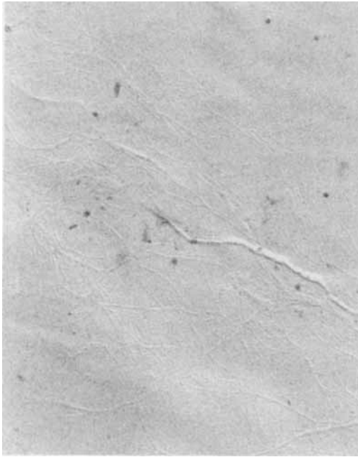
FIGURE 2 Fibrils of P Layer of Fiber Replica x10000
