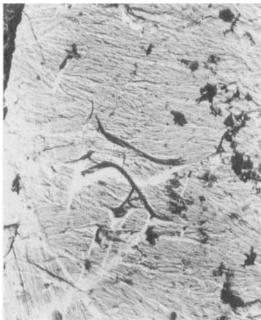
FIGURE 3 Fibrils of S_1 Layer in Fiber Replica x10000
